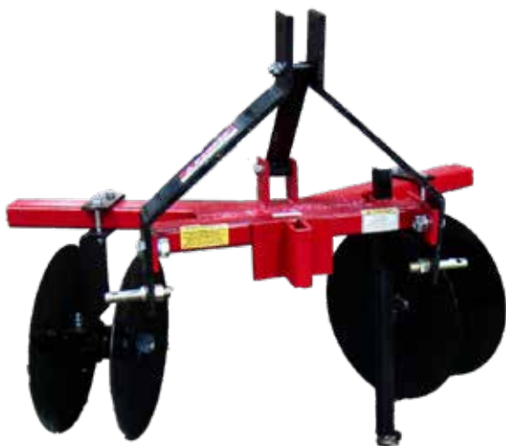
Compact Cat 1 3Pt hitch Hiller/Ripper
